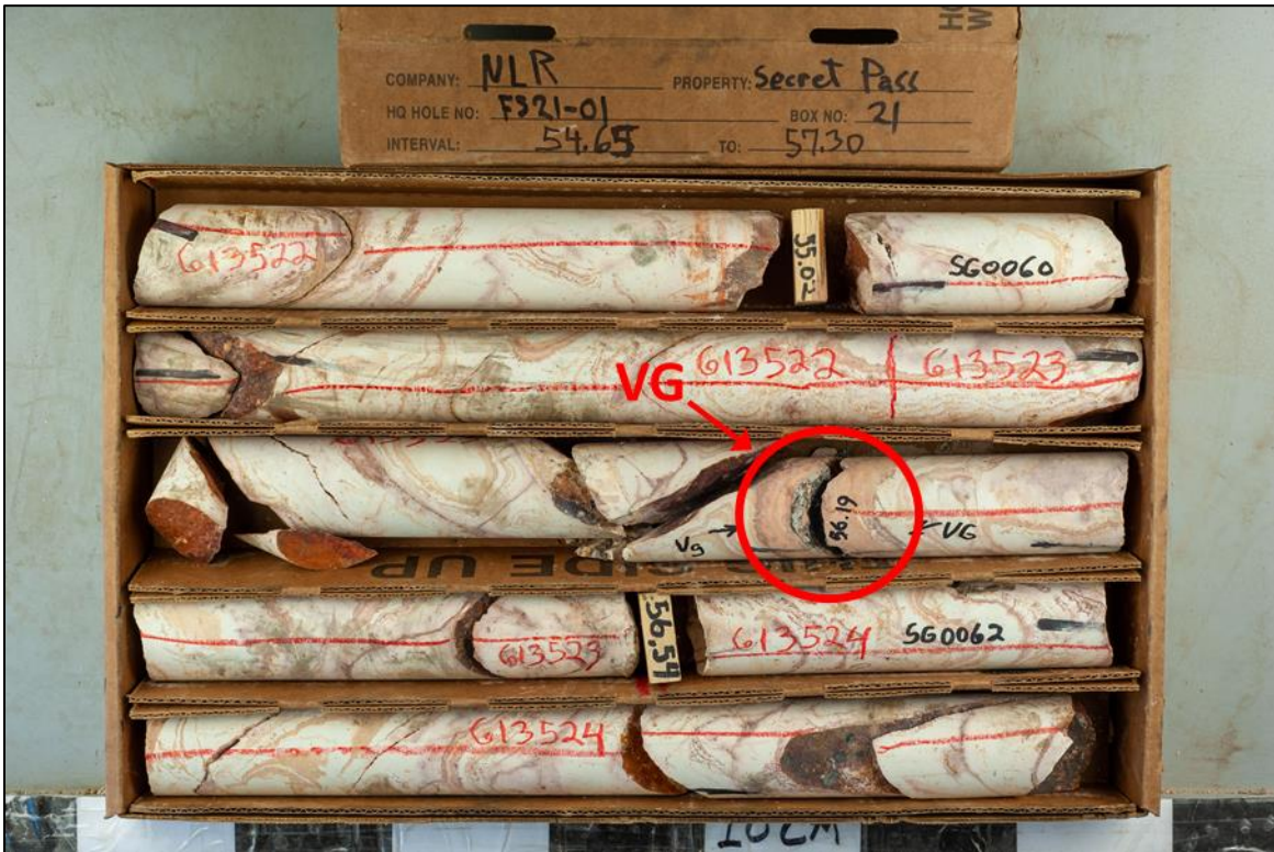
Figure 2: FS-02 Drill Core showing VG intersection at 56.2 metres hole depth
