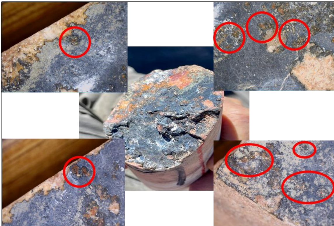
Figure 1: FS-02 Drill core (size HQ approximately 75 mm diameter) showing Visible Gold along joint plane (VG shown in red circled locations)
